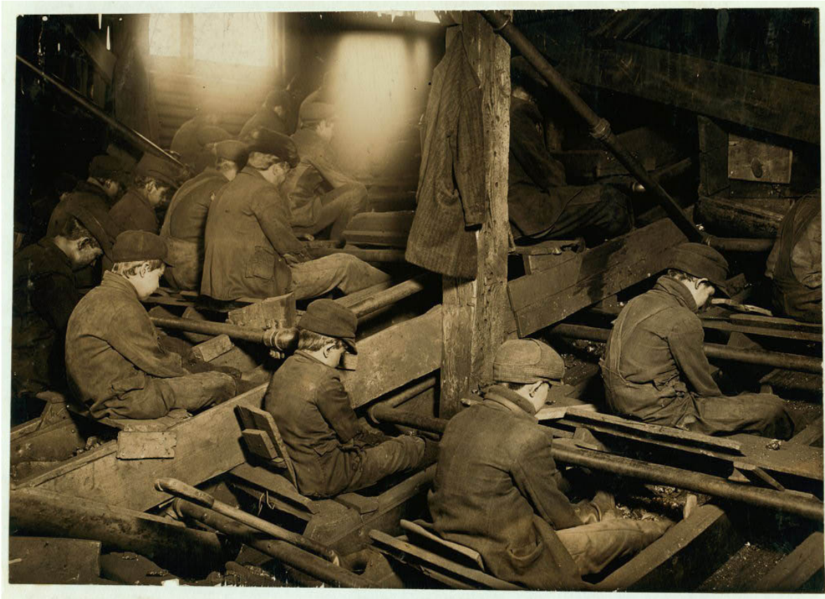
Breaker boys separated coal from rocks or other debris. This work was done above ground but still posed hazards to young workers. They sat in a room dark from the thick coal dust for hours. Just like the children working underground, breaker boys inhaled great amounts of coal dust damaging their lungs and causing illness. Breaker boys handled thousands of pieces of coal each day and the sulfur on the coal would cause their fingers to swell and bleed. The sounds of the machines used were deafening and able to crush small hands quickly.
