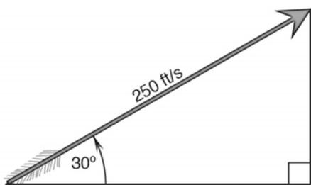
In order to do this problem we need to figure out how long the arrow will be in flight. The primary force limiting the arrow's travel is gravity (since we are ignoring air resistance). Gravity is what will push the arrow back down and into the ground. Gravity only operates vertically. Gravity has no effect on the horizontal progress of the arrow. So it is the gravity that determines how long the arrow will be aloft. To determine this we use one of the kinematic equations:
